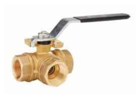
3-way brass ball valve, 4 seated T port (3T-3300) or L (3L-3400), threaded-in end caps, ISO 5211 direct mount actuator pad, locking handle
