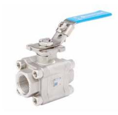
3-piece 2000 CWP carbon or stainless steel ball valve, API 607 fire tested (standard), ISO 5211 direct mount actuator pad, locking handle, tongue & groove body seal, spring loaded packing, in-line maintainable
